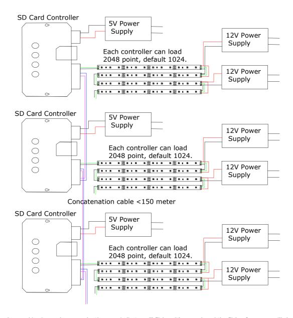
Note: when working in synchrony mode, the error indicator will flicker, it's normal, and the flicker frequency will change when working in different speed. (The first DMX controller doesn't flicker, otherwise its wrong).
